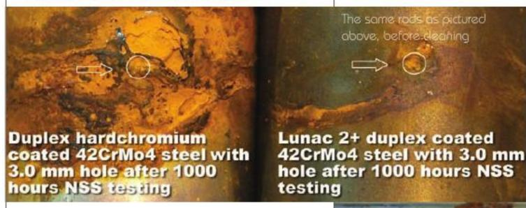
smooth (Ra 0.11-0.3  $\mu$ m) and the coating will not peel off even after a plastic deformation, however the top layer of the Lunac +2 can show microscopic cracks if stretched more than 0.28 per cent. Lunac 2+ duplex is designed to withstand the harshest of environments.
